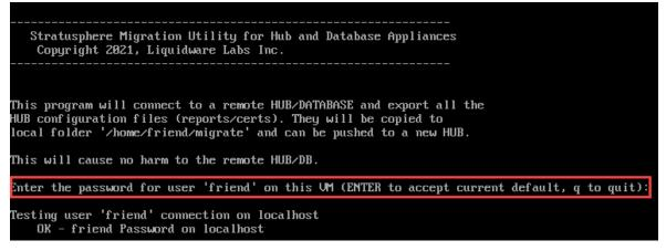
The wizard will then prompt to enter the IP address of the remote (old 5.8.6 or higher) Stratusphere Hub. It will then test to see if the default credentials for **friend** and **root** users can be used to connect to the remote (old 5.8.6 or higher) Hub. If not, it will prompt the user to enter the **friend** and **root** credentials.
